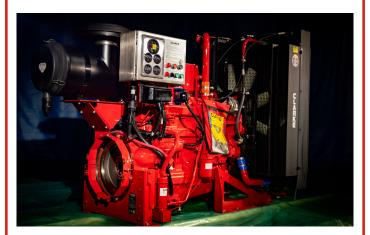
Radiator cooled engines have coolant that is sent to the radiator. The coolant flows through tubes that penetrate through the fins. An engine driven fan blows air across the radiator fins, which then removes the heat from the coolant. The coolant then travels back to the engine block through the engine water pump and the cycle continues while the engine is running.
